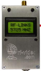
New Microwave Transmitter model WTX-5800 is a fully synthesized audio/video transmitter for wideband frequencies from 5600 MHz- 5900 MHz. It is a Military grade unit that covers the wide frequency range. The RF power output power is 10 mW or 100 mW (Model WTX-5800/H. It sends a crisp color picture and sound miles away. No special tuning is needed. Simply choose the frequency with two push-button switches. Digital display shows desired frequency. Antennas are not included.
