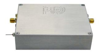
The new wideband linear amplifier for UHF band based on single IC chip is an excellent design made for special applications, lab testing, digital and analog RF and TV applications. Amplifier model WFL-25 covers entire band VHF-UHF from 30 MHz- 2.5 GHz. This board requires 28 VDC / 0.5 A. The minimum driving input is 30 dBm; required RF input for the maximum RF output power is 32 dBm. Rated output RF power is 10 W max.
