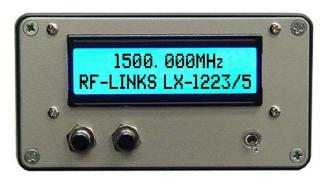
The new Audio/Video transmitter is a special design for Military applications capable to work in extremely low or high temperature range. This transmitter has wide range of frequencies from 1200 MHz- 2300 MHz with no gaps or limits. This transmitter has digital display. It is easy to change channels using 2 push buttons Up / Down. This transmitter has 5 W RF power thank to special wideband circuitry. LX-1223/5 works from 9 V- 16 V.
