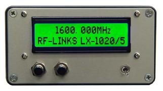
The new Audio/Video transmitter is a special design for Military applications capable to work in extremely low or high temperature range. This transmitter has wide range of frequencies from 1000 MHz- 2000 MHz with no gaps or limits. This transmitter has digital display. It is easy to change channels using 2 push buttons Up/ Down. This transmitter has 5 W RF power thank to special wideband circuitry. LX-1020/5 works from 9 V- 16 V.
