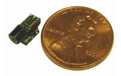
This is the ultra small newest CMOS Color Video camera with built-in video transmitter. This small combo will give you an excellent picture quality. This combo is available in 2.25 GHz band using special receiver. Complete camera with transmitter takes 28 mA / 3V from watch battery. Dimensions: 0.35" X 0.19 " X 0.25"
