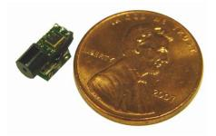
This is the ultra small newest CMOS Color Video camera with built-in video transmitter. This small combo will give you an excellent picture quality. This combo is available in 1.9 GHz band using special receiver. Complete camera with transmitter takes 28 mA / 3V from watch battery. Dimensions: 0.3" X 0.19 " X 0.2" or 9 mm x 4.8 mm x 5.5 mm
