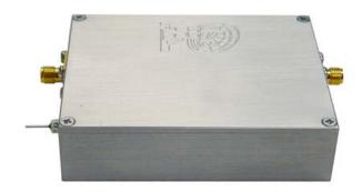
This is a high quality professional 15 W linear amplifier that requires minimum driving input of only 1 m W for the maximum of 15 W RF power output in 900 MHz range. This amplifier is linear and doesn't require any tuning or adjusting. Power supply is 12 V/2.6 A. Gain is 30 dB. Input / Output impedance 50 ohms. This amplifier has built-in band pass filter for 900 MHz band.
