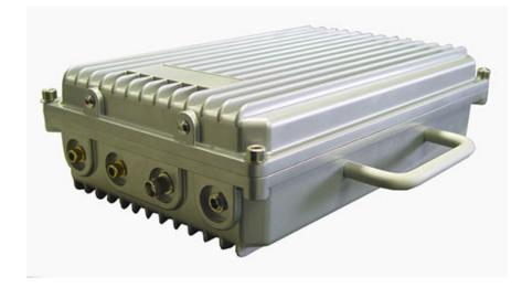
Model AMP-50PBS is a professional TV linear amplifier in AB class with 50 W RF output power and 50 mW input power. It is recommended as a driving amplifier for high power stages or small TV stations. This linear amplifier works from 760-870 MHz and it is perfect for Analog or Digital TV broadcast applications. Gain is 26 dB. Fully mobile this amplifier has been built in an outdoor, weatherproof box. Output connector is N female type.
