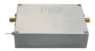
This is a high quality Professional VHF TV linear amplifier module broadband from 350 MHz- 520 MHz. This amplifier needs only 5-25 mW RF power for 7 W output. Power supply requires DC voltage 12 V /1.6 A. Extremely linear this amplifier has been made for small TV stations and studios. It is ideal as an exciter for high power TV stages and digital applications. Warranty one year is included. This amplifier must be installed on a heat sink (not included).
