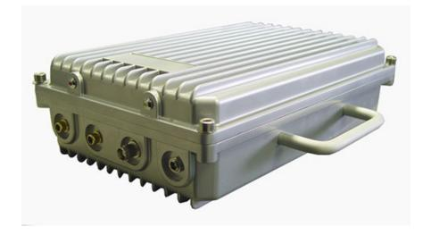
Model AMP-150PBS is a professional TV linear amplifier in AB class with 150 W RF output power and 2-4 W of input power. It is recommended as a driving amplifier for high power stages or small TV stations. This linear amplifier works from 470-860 MHz and it is perfect for Analog or Digital TV broadcast applications. Gain is 16 dB. Fully mobile this amplifier has been built in an outdoor, weatherproof box. Output connector is N female type.
