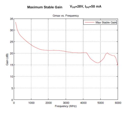
**Typical Performance: Gain, Efficiency and Output Power**
