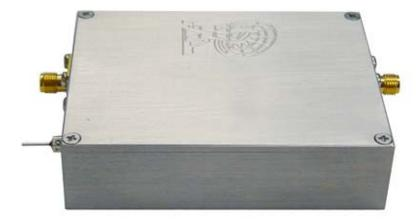
This is a high power broadband amplifier for labs or testing purposes. This amplifier is excellent for SUHF band 10 MHz - 6000 MHz. The gain is over 40 dB. The maximum power is 5 W. Minimum required driving power is only 1 mW. This amplifier is recommended for Space research, Mil applications etc. Dimensions: 3.25 " X 2.5 " X 0.8 ".
