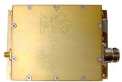
This is a high power broadband amplifier for labs or testing purposes. This amplifier is excellent for SUHF band 10 MHz - 6000 MHz. The gain is over 40 dB. The maximum power is 10 W. Minimum required driving power is only 1 mW. This amplifier is recommended for Space research, Mil applications etc.
