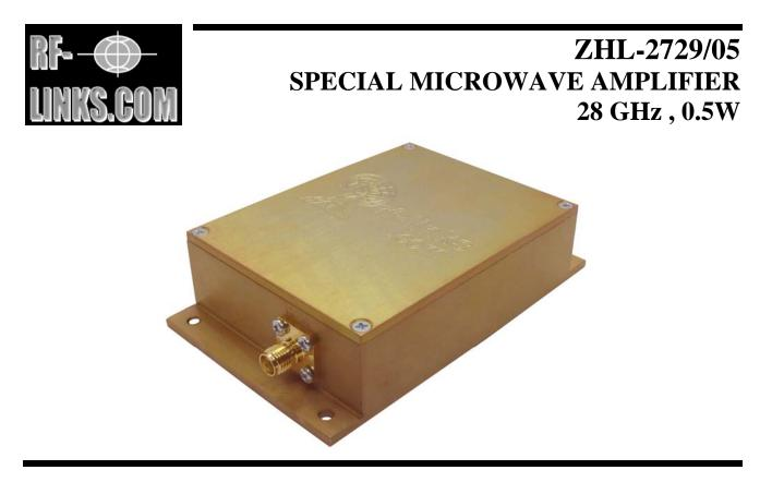
This power amplifier for 28 GHz is based on a  $0.15\mu$ m pHEMT technology, which allows a very high output saturation power of 0.5W typically. All internal bias voltages are generated from a single 12 V supply voltage, which is used efficiently by means of a switching regulator. Also, there is an over temperature shutdown implemented.
