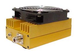
This is a tested high quality professional 20 W RF amplifier that requires minimum driving input of -5 dBm for the maximum of 20 W RF power output. Driving Input of 0 dBm will give 30W RF Output power. It is broadband in 880 MHz- 960 MHz and doesn't require any tuning or adjusting. Power supply is 12 V/6.8 A max. Gain 26 dB. BNC / N female connectors Input / Output 50 ohms impedance. Class of operation AB.
