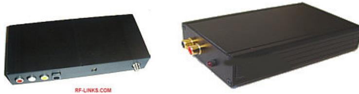
XL 2000/M is a portable microwave link. It is frequency agile in 2.4 GHz band. XL 2000/H is excellent solution for mobile applications and TV broadcast transmission up to 6 km line-of-sight.
