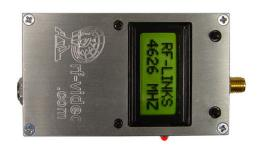
New Microwave Transmitter model WTX-4466 is a fully synthesized audio/video transmitter for wideband frequencies from 4400 MHz- 6600 MHz. It is a Military grade unit that covers the wide frequency range. The RF power output power is 10 mW or 100 mW (Model WTX-4466/H. It sends a crisp color picture and sound miles away. No special tuning is needed. Simply choose the frequency with two push-button switches. Digital display shows desired frequency. Special omni directional antenna is not included.
