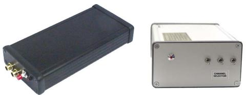
This is the long range microwave system 5.8 GHz 5 W RF power, tested for long distances over 40 miles from the air with special high gain antennas. The new system includes transmitter, receiver, antennas are sold separately.
