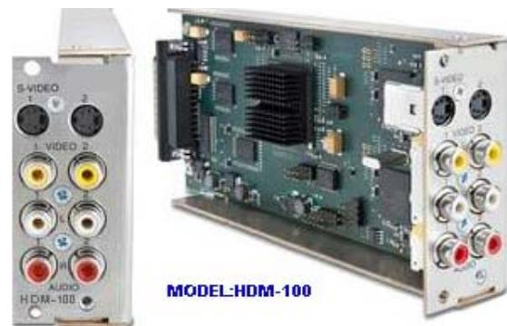
Each HDM-100 module provides two sets of input connectors for NTSC composite or S-video with stereo audio. Audio is encoded using Dolby AC-3 encoding.
