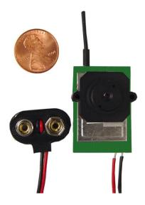
This is the ultra small newest CMOS Color Video camera with built-in video transmitter. This small combo will give you excellent picture quality. This combo transmits in 5.8 GHz band using our matching receiver. Complete camera with transmitter takes 118 mA / 9 V. Dimensions: 0.9" X 1.5 " X 0.8"
