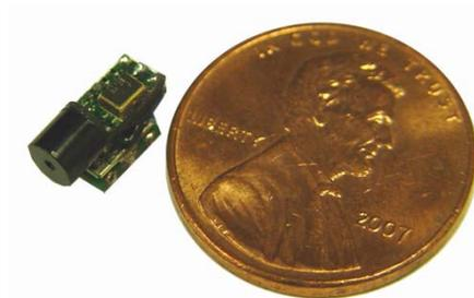
This is the ultra small newest CMOS Color Video camera with built-in video transmitter. This small combo will give you an excellent picture quality. This combo is available in 2.25 GHz band using special receiver. Complete camera with transmitter takes 28 mA / 3V from watch battery.
