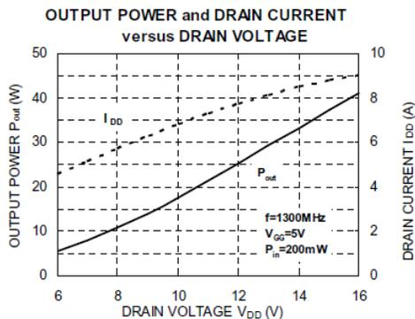
**TYPICAL PERFORMANCE** ( $T_{case}=+25^{\circ}C$ ,  $Z_G=Z_L=50\Omega$ , unless otherwise specified)
