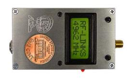
This special Wideband receiver will give you opportunity to monitor any frequency from 4950 MHz- 6200 MHz. Fully synthesized this World's smallest Microwave receiver is perfect for monitoring high frequency video band. It is fully portable, extremely sensitive and easy to use. You can simply press UP/DOWN button to change the frequency. This wideband receiver
