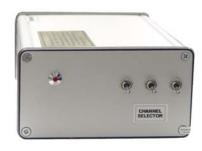
This special Wideband receiver will give you opportunity to monitor any frequency for 4950 MHz band in 8 channels. Fully synthesized this system is perfect for transmitting high frequencies from the flying vehicle. It is fully portable and easy to use system. Antennas for this system are sold separately.
