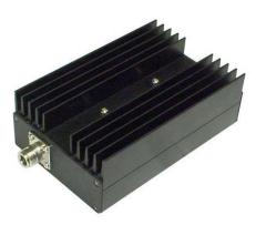
The new 1.7 GHz Audio/Video transmitter is a special design for Military applications capable to work in extremely low or high temperature range. This transmitter has 8 easy to change channels and 10 W RF power. This video transmitter works from 12 V-16 V.
