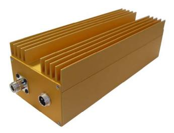
This extreme rugged HIGH GAIN power amplifier has been designed to cover the entire HF band from 1 to 30 MHz, offering unsurpassed solution for HF power amplifier designs. Designed for CW applications, the ZH-0114/200 is equipped with the latest generation of LDMOS super rugged power devices for extreme reliability required by military tactical and heavy duty civil RF equipment. (Blowing fan needed.)
