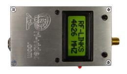
This special Wideband receiver will give you opportunity to monitor any frequency from 4400 MHz- 6600 MHz. Fully synthesized this World's smallest Microwave receiver is perfect for monitoring high frequency video band. It is fully portable, extremely sensitive and easy to use. You can simply press UP/DOWN button to change the frequency.
