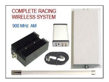
900 MHz complete wireless TV system S-900 is an excellent solution for car racing. It comes with a high power video transmitter 10 W, receiver RM-900B, dipole antenna and panel antenna 8 dB gain. This system is excellent to send a broadcast quality video signal over 16 km. The range in open area is much greater. This system is available in 2 different channels.
