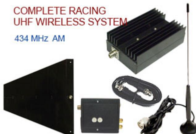
UHF complete wireless TV system S-430 is an excellent solution for car racing. It comes with a high power video transmitter 10 W, receiver M-806, shark fin antenna and magnet mount antenna 3 dB gain. This system is excellent to send a broadcast quality video signal over 10 km.
